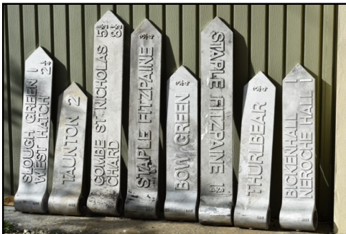
8 new raw castings back from the foundry
