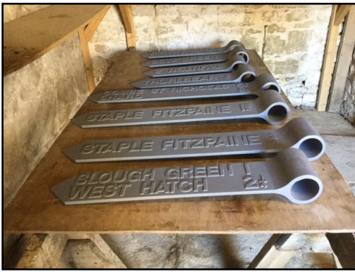
Primed arms in storage ready for painting
